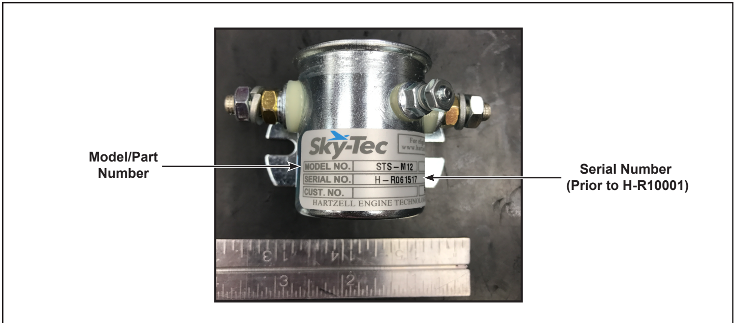
Affected Master Contactor. Model Number STS-M12 Shown. Figure-1
