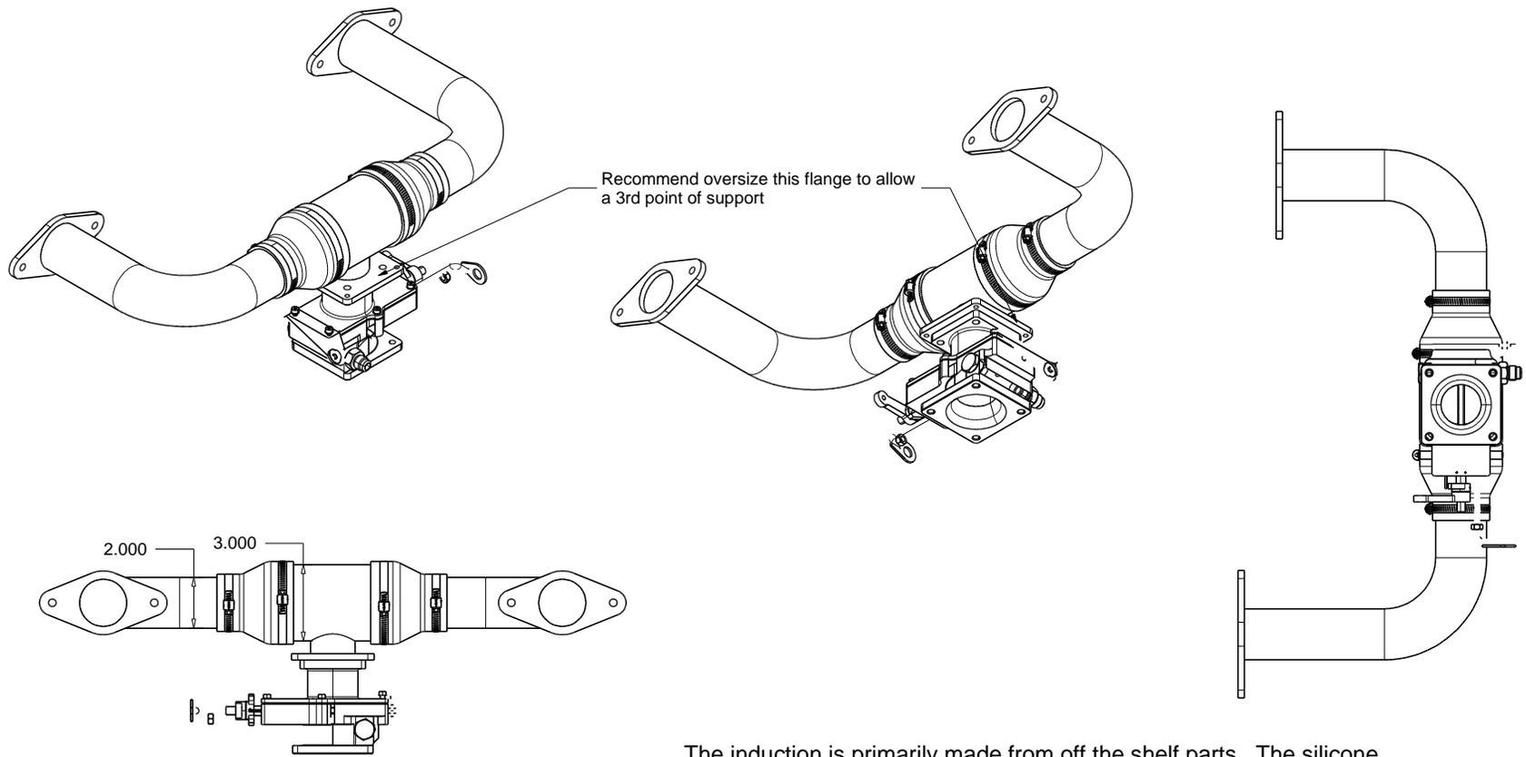
The induction is primarily made from off the shelf parts. The silicone reducers and 2" aluminum elbows are available online. The legs of the 2" elbows can be cut to fit the needs of the particular installation.
